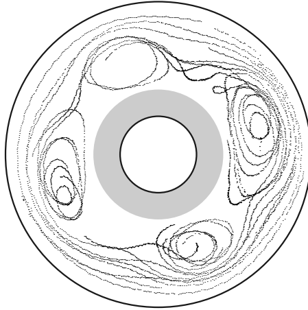
Fig. 4. The four-vortex flow is revealed by the trajectories of 12 particles tracked for 100 s in a reference frame co-rotating with the vortices. The inner and outer circles represent the annulus boundaries, and the grey circle indicates the location of the Plexiglas barrier. (Figure from Ref. [12].)
